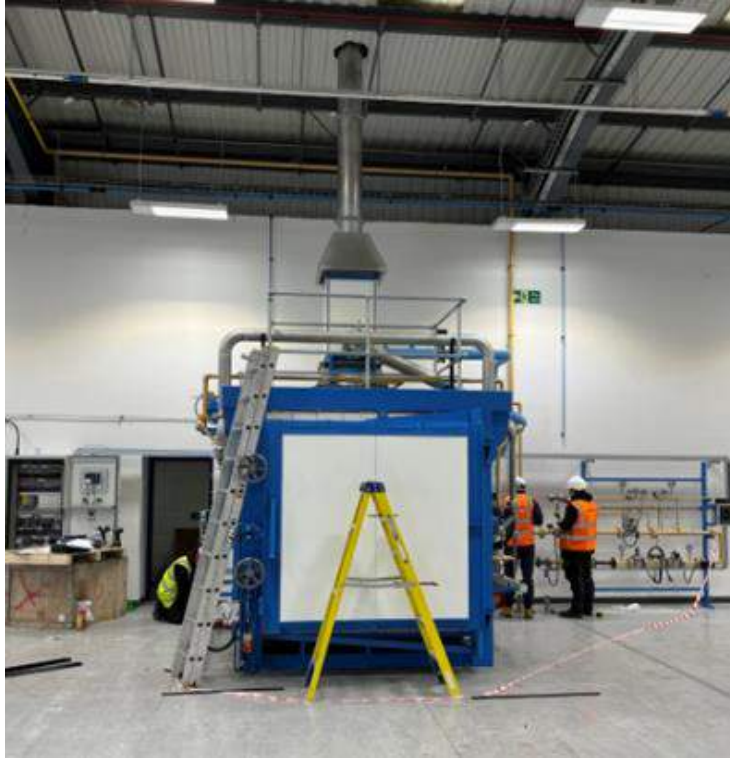
Batch research kiln fitted for 100% H2 up to 1750°C, commissioned by May 2024
