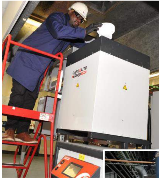
Electrolytic metal refining pilot rig (can mimic EAF)
