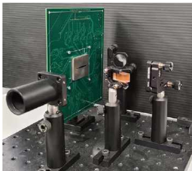
Above: Ultra low cost mid-wave infrared spectrometer.
