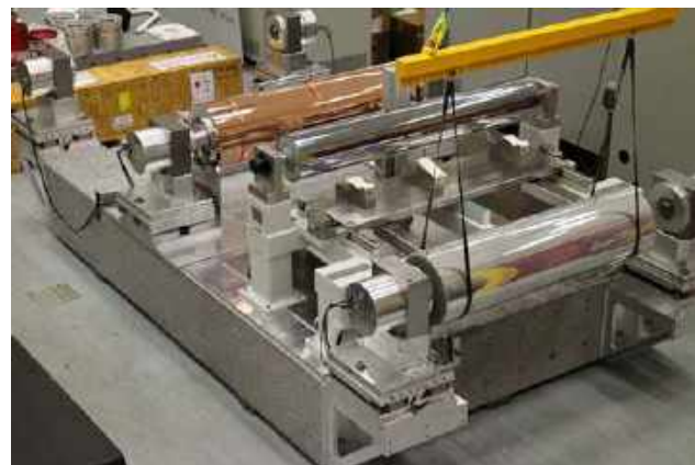
Above: Fast THz optical sensor with roll-to-roll system demonstrator.
