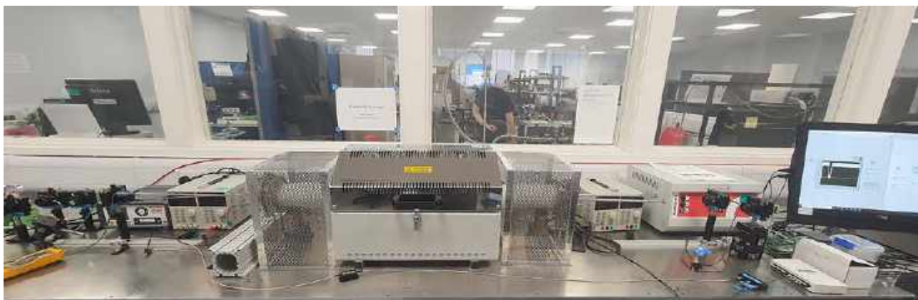
Above: Dual radiometer setup with split-tube furnace.
