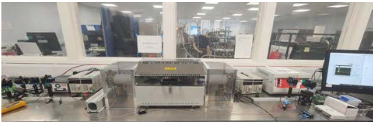
Above: Dual radiometer setup with split-tube furnace.
